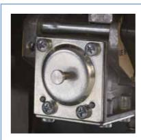
Enerkit Each Water Pump is equipped with a unique LPG dedicated ENERKIT carburettor, allowing optimum performance. ENERKIT has an automatic safety shut off valve, stopping the fuel supply when the engine is off.
